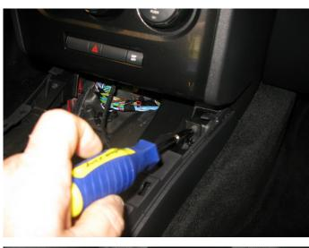
**Step 6:** Pull the radio bezel off and, using the 3M wire taps provided, tap into the following wires that are in the harness that leads to the ESP button: Ground (black or grey) from the NO-ESP board taps into the (black/light green stripe) wire on the harness. The ESP (green) wire taps into the (dark green/white stripe) wire.
