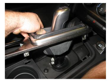
**Step 2:** Remove the upper center console half. This also just pulls up. There is a harness attached to the lighter outlet, so you will have to disconnect it.
