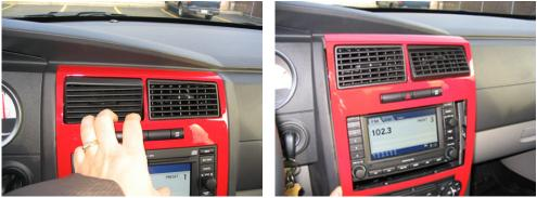
**Step 2:** Pull out the shifter tray. Insert finger in hole on side of bezel(in the tray area) and pull up on bezel to pop the snaps. Do not pull up on the front of the bezel, as it is still held in place by two screws near the ash tray.
