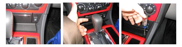
**Step 4:** Disconnect the wire to the radio bezel and set the bezel aside. Pull the ash tray out. Remove the wiring to the cigar lighter, and seat heat switches, if equipped.
