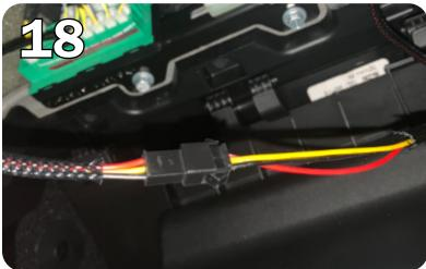
Pull the male connector of the mesh harness behind the glove box from inside it and reconnect the male and female halves of the harness.
