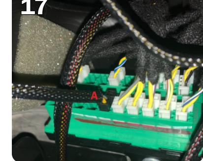
Plug the CAN connector into the STAR connector behind the glove box. (A)
