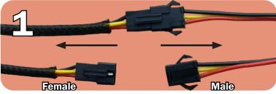
• The half with the male connector ends in the connectors that will connect to the relay board.
