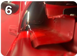
Open the front passenger door to reveal the throughhole where the male connector attached to the rod will be snaked through.
