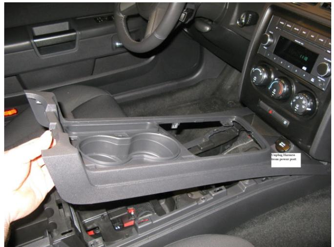
**Step 3:** Remove the two Philips screws that hold the front of the center console in place.
