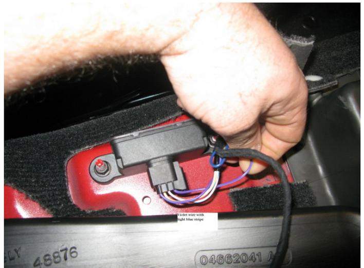
**Step 6:** Pull the radio bezel off and, using the 3M wire taps provided, tap into the following wires that are in the harness that leads to the ESP button: Ground (black or grey) from the NO-ESP board taps into the (black/light green stripe) wire on the harness. The ESP (green) wire taps into the (dark green/white stripe) wire.
