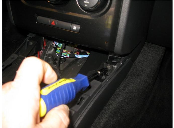
**Step 4:** Remove the (4) 8mm bolts that hold the rear of the center console in place. The console can now lift out of the way, or simply be slid back for access.
