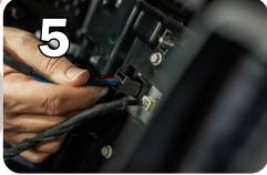
Pull or pry up the trim that sits below the passenger's side door and to reveal the STAR Connector.  Unplug the connector by pressing the tab and pulling straight out.
