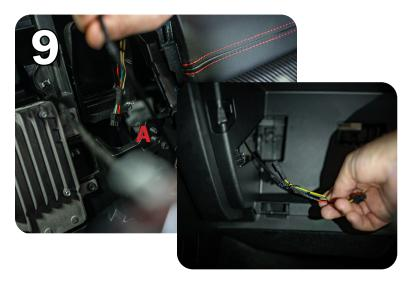
Thread the wire harness into the hole in the plastic panel at the back of the compartment (A) all the way to the opening on the right (B).
