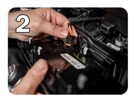
Plug the connector into the matching female end on the kit's wire harness.
