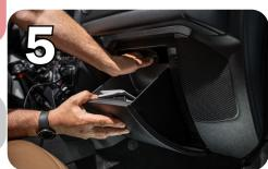
Pass the 6-pin connector through the opening to the right behind the HVAC panel into the glove box and pull it through.
