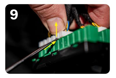
Plug the connector into the matching female port on the NoLimitz wire harness.
