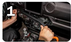
Unplug the connector by pressing the tab and pulling straight out.
