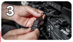
Plug the male connector on the wire harness into the HVAC control panel and set it aside.
