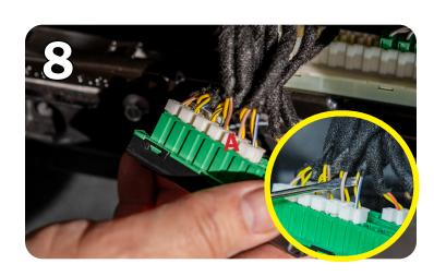
Remove the connector by wedging a flathead screwdriver into the gap above the green plastic to depress the latch and pull straight out.
