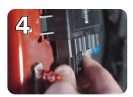
Connect the ParkSense Fix electronics module to the wire harness.
