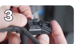
Connect that plug to the female connector on the kit's wire harness.
