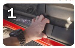
Disconnect the nearest plug in the ParkSense Module by depressing the tab and pulling straight down. (A)
