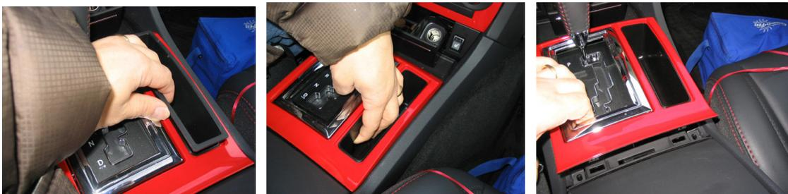
**Step 3:** Remove the cover in front of the ashtray. This simply pulls up. Underneath are two Philips head screws to remove.
