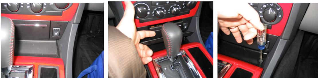
**Step 4:** Disconnect the wire to the radio bezel and set the bezel aside. Pull the ash tray out. Remove the wiring to the cigar lighter, and seat heat switches, if equipped.
